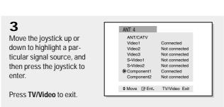
When you press the TV/Video button, the on-screen display identifies all the active video sources (and their corresponding input jacks):
